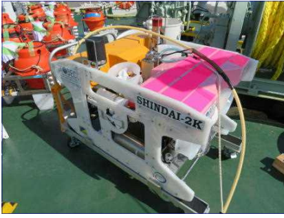
ROV遠隔操作水中探査システム (Remotely Operated Vehicle)
