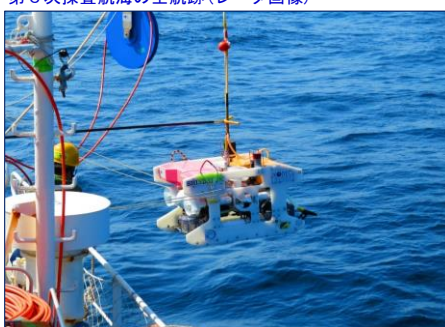
ROV (Remotely Operated Vehicle) 遠隔操作水中探査機
